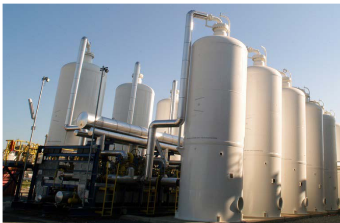
Figure 3: 12-bed Polybed PSA (Belgium)
