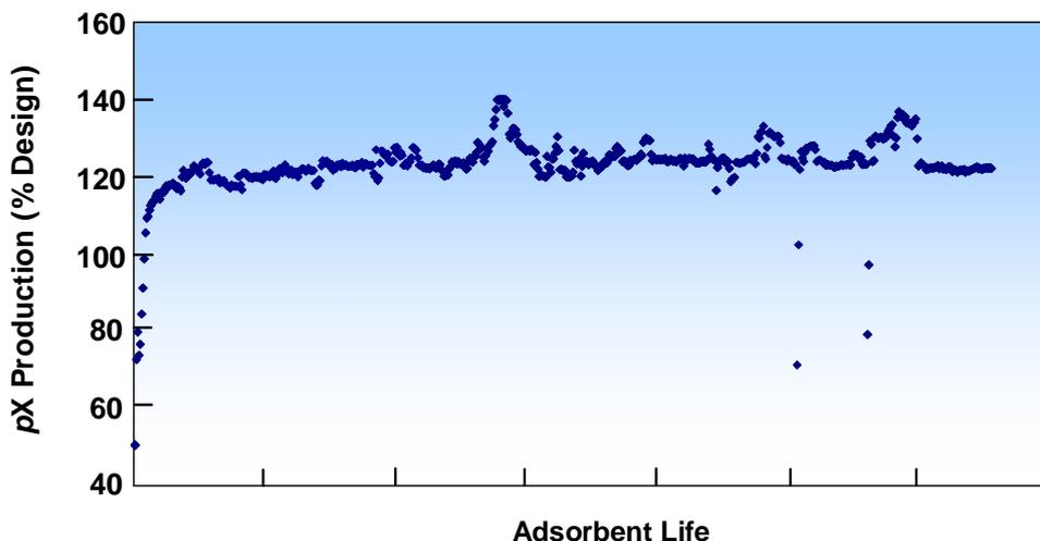
The performance of ADS-37 adsorbent at this facility has also been extremely stable at this high operating capacity, with target product purity of greater than 99.7 wt% at more than 98% recovery over the 2+ years this adsorbent has been in service, as seen in Figure 5.
