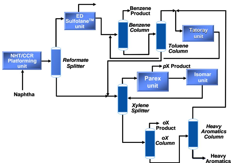
The Parex Process, the key to the production of high purity *para*-xylene, uses a selective and proprietary solid adsorbent developed by UOP to separate *para*-xylene from a mixed C<sub>8</sub> aromatic stream. Commercial Parex Process units typically are able to produce 99.9 wt% *para*-xylene purity at greater than 97% recovery.
