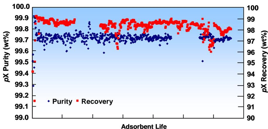
Since 2004, the improved performance of ADS-37 adsorbent has been demonstrated in several commercial Parex units. By the end of 2006, a total of 11 commercial Parex units were operating with ADS-37 adsorbent. This substantial and immediate acceptance by the marketplace has resulted in 16% of the world's current *para*-xylene being produced with ADS-37 adsorbent, as is shown in Figure 6.
