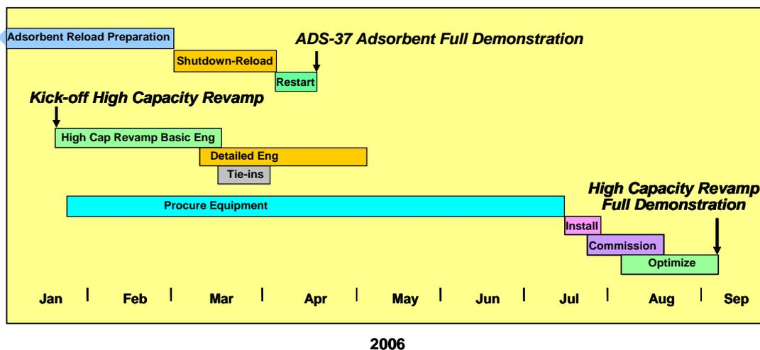
The basic engineering was completed, and ATC then had its contractor complete the EPC work. The shutdown to load ADS-37 adsorbent went as planned, and all tie-ins required for the high capacity revamp were made during the shutdown. By early April 2006 the plant was back on-stream, achieving approximately 6% additional capacity because of the ADS-37 adsorbent.
