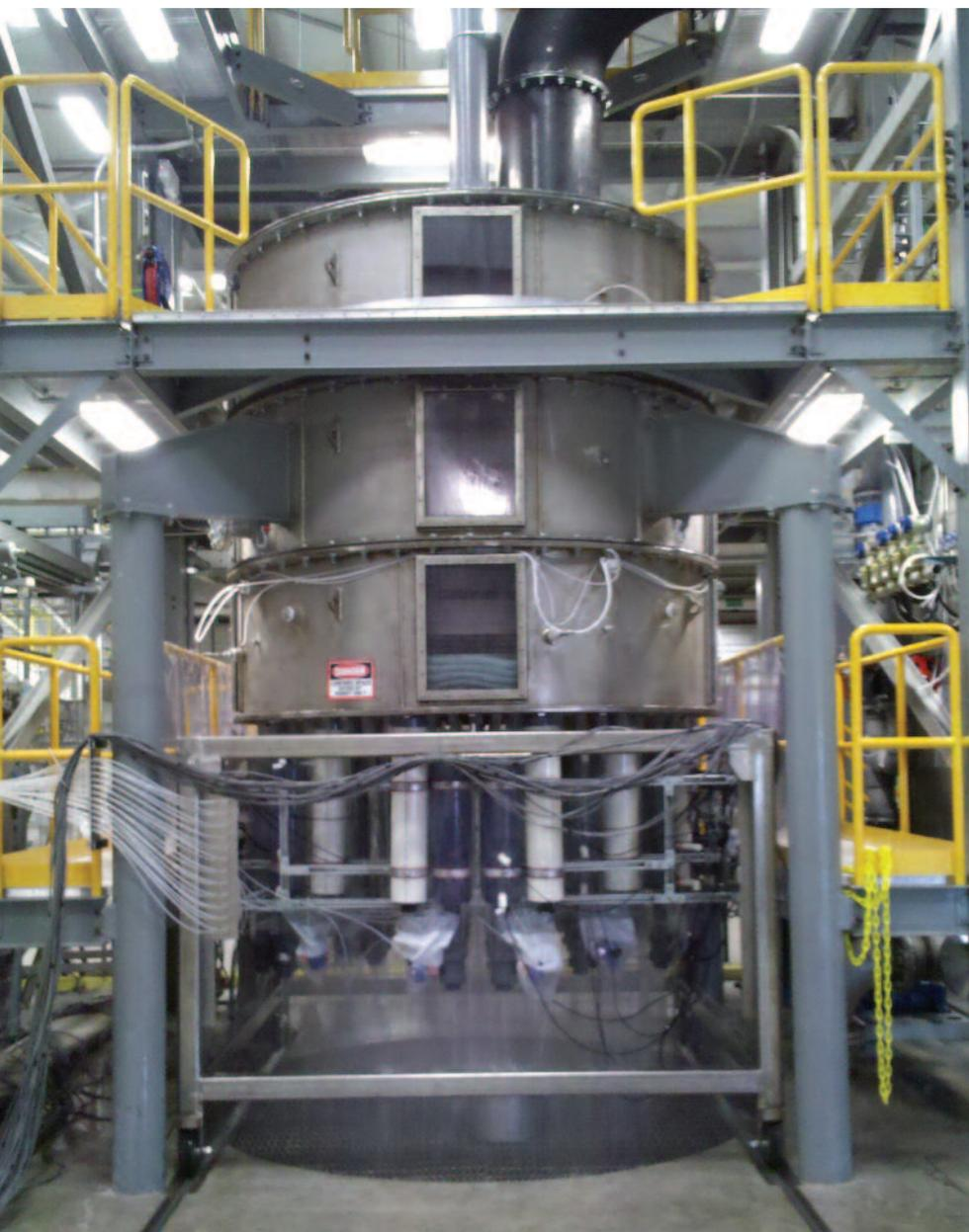
**Figure 2** Cold flow test column Source: UOP
