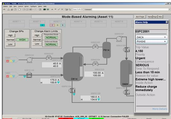
Figure 3: Alarm Help from Experion Operating Graphics
